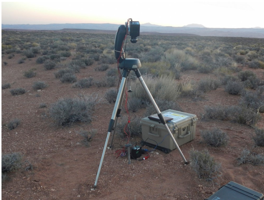
Figure 2: A typical National Park Service Night Skies Program camera system consists of a commercial lens, a V-band filter, and a CCD camera. The camera system is mounted on a motorized mount, hooked up to external batteries, and controlled by a computer.
